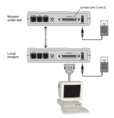
Figure C-5. Back-to-back test connections.
